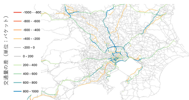
Fig. 1 Nationwide-scale simulation calculating traffic volume changes by toll changes (Tokyo area enlargement)
