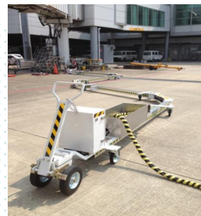
Electric cable container
