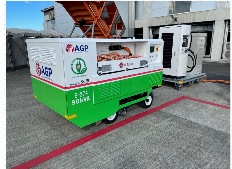
Battery-powered GPU Dimensions L2,745 x W1,480 x H1,620mm Weight 2,200KG Less than
