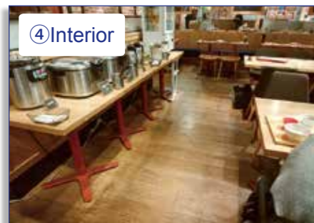
④ Interior Enough turning space for wheelchair Aisle width - 110cm
