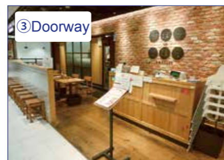
③ Doorway Open entrance with no steps Entrance width - 180cm
