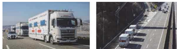
Realization of unmanned platooning of following vehicles (February 2020)
