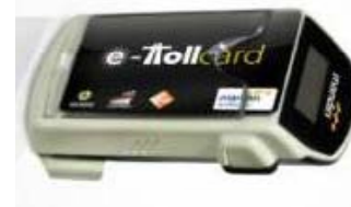
e-Toll pass On Board Unit provided by Bank Mandiri is based on Malaysian National Standard
