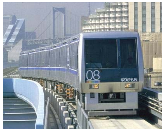
Sistema de Trânsito Guideway Guideway Transit System
