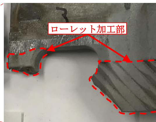
(c) 孔縁端部の破断 (支柱④)
