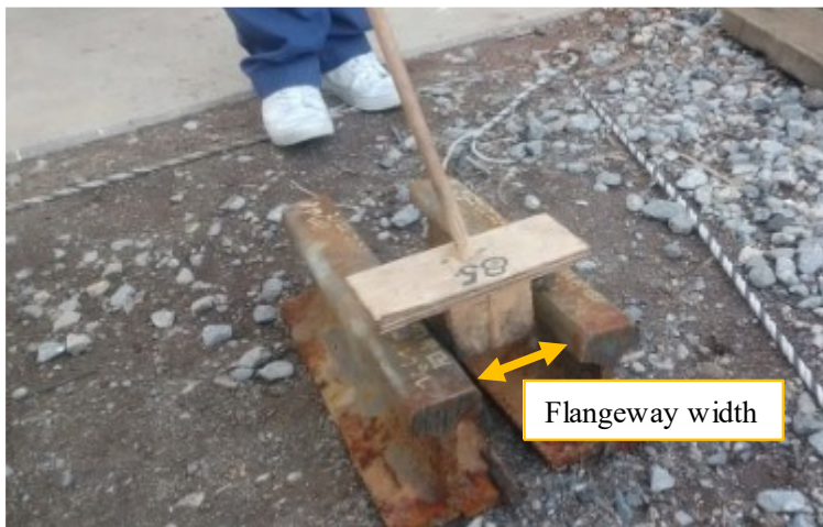
Figure 5. Measuring Tools for Flangeway Width
