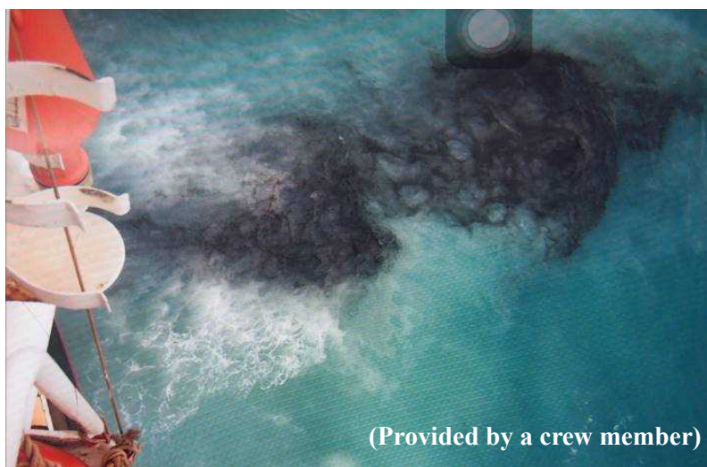
Photo 4 Fuel Oil Leaking from the Vessel's Stern
