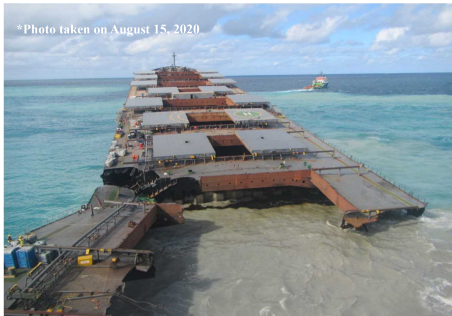
Photo 7 The Vessel's Bow Separated from the Stern
