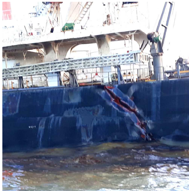
Photo 11 Fuel Oil Spilling from the Rupture
