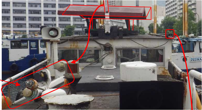
State of damage to the mast, starboard light, wheelhouse, etc. (Taken from the stern side)
