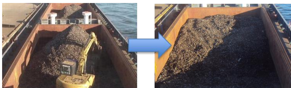
Photo 2.5-2 Leveling of Shredded Scrap in a Cargo Hold (Photos provided for conceptual purposes.)
