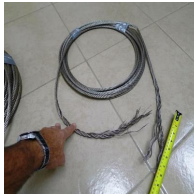
Photo 5: Broken state of this wire rope
