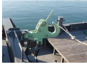
Photo 7: Hook after Replacement (with emergency breakaway device)
