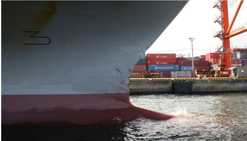
Photo 4 Damage to Vessel A's Starboard Side
