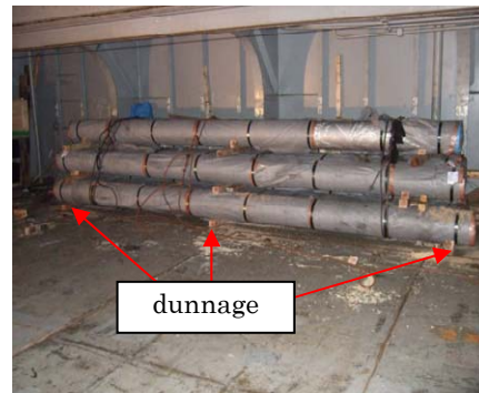
Photo 2.1-3 Laying of dunnage 2
