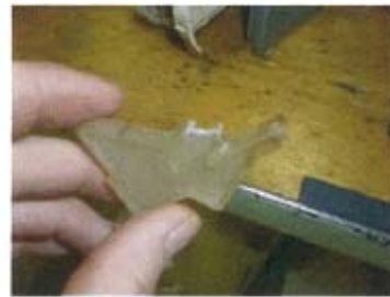
Damage to a plastic part in the internal linkage mechanism
