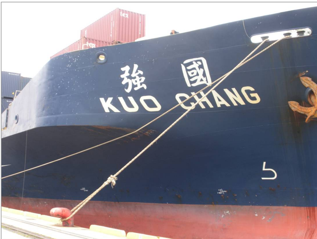
Photo2: Forward Spring Line (Kobe District, Taken at Hanshin Port)
