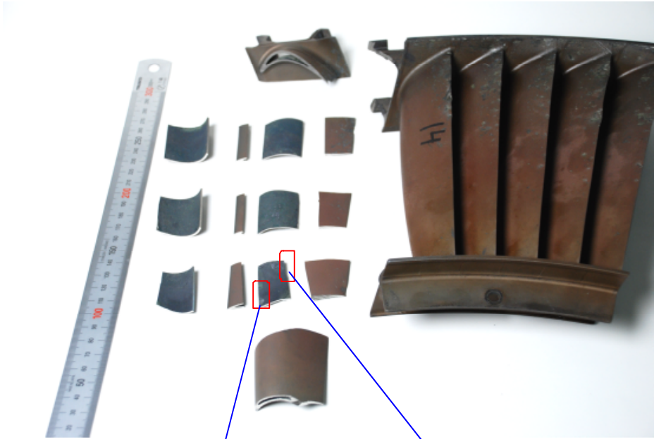
Photo 9 Intergranular Corrosion and Intergranular Oxidation of LPT STG-2 NGV Inner Wall Surfaces
