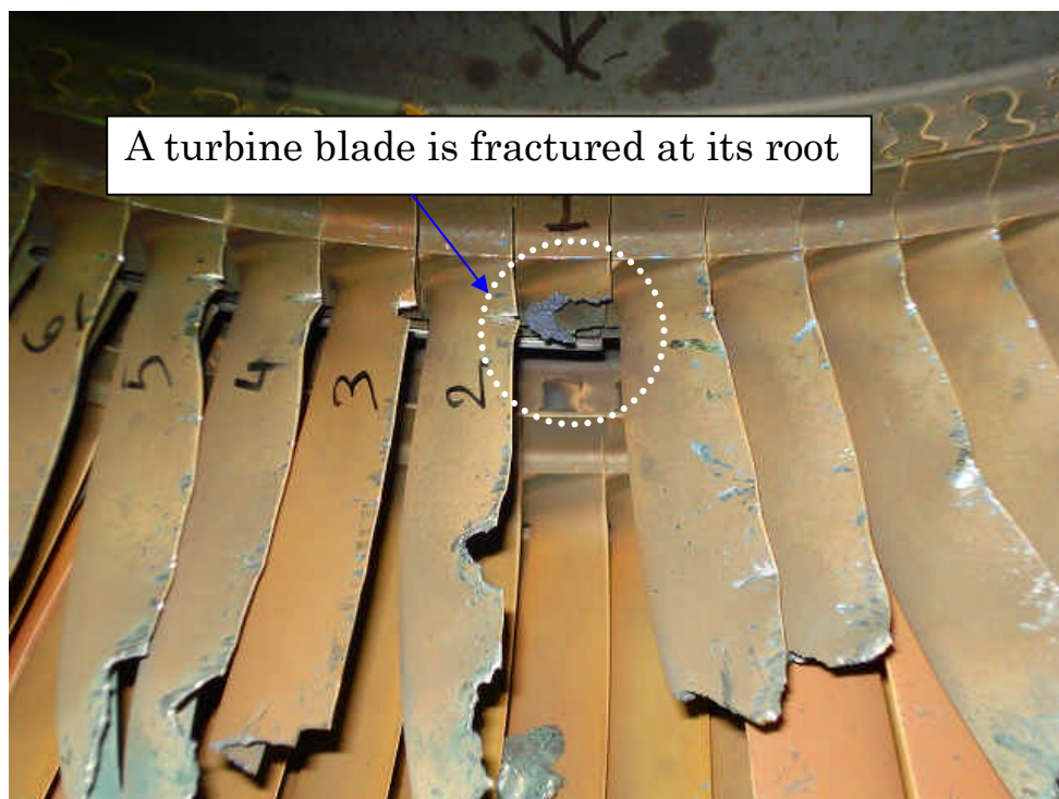
Photo 4 Fractured Turbine Blades of LPT STG-2
