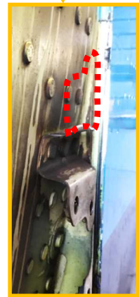
A bracket that broke and remained on the fuselage side
