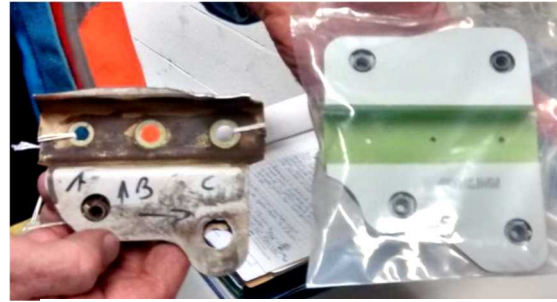
Broken bracket Enhanced design bracket
