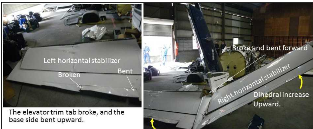
Figure 15: damage to the horizontal stabilizer
