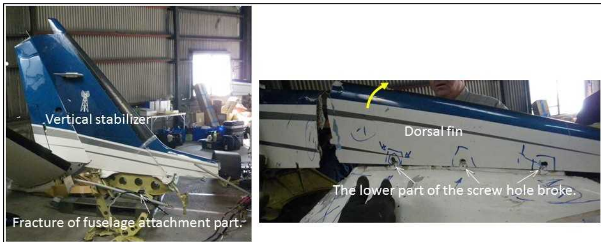
Figure 16: damage to the vertical stabilizer
