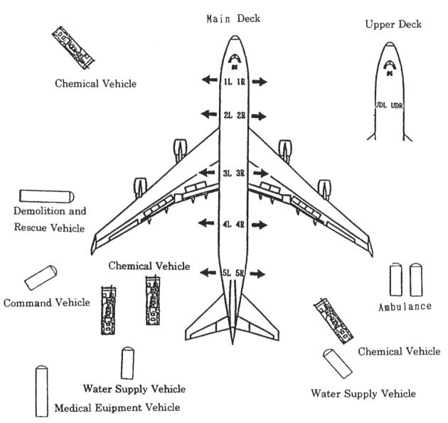
Note: 1 Arrows ( $\leftarrow \cdot \rightarrow$ ) in the drawing show the deployed evacuation exits.
