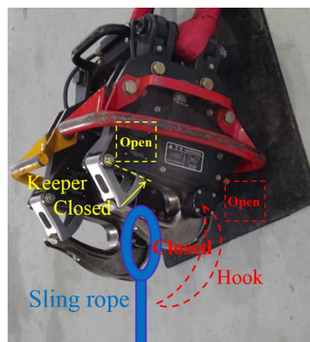
Fig. 1 Cargo hook with slung cargo, opening and closing (conceptual diagram)
