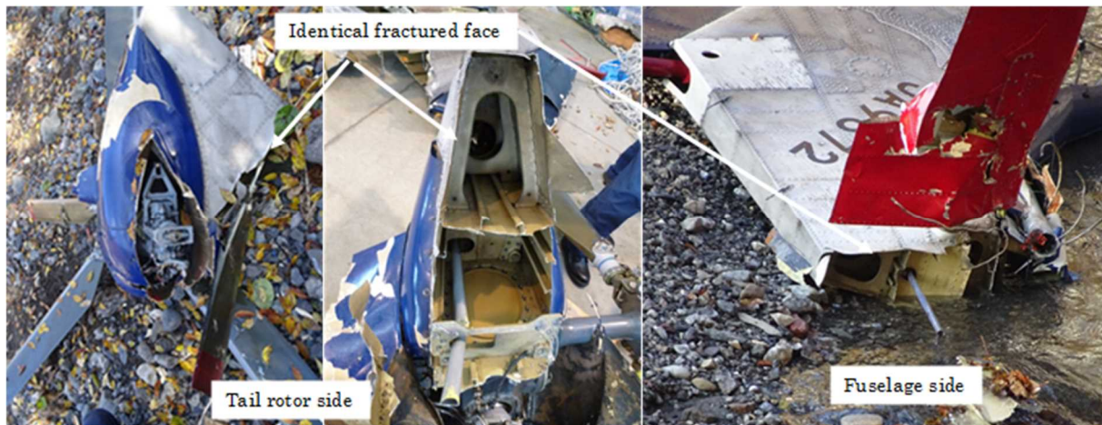
Figure 32: Fractured face of tail rotor lower side separated from airframe
