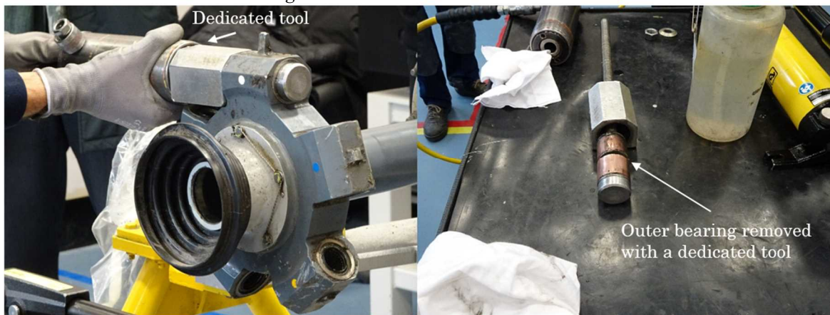
Figure 25: Outer bearing removed with a dedicated tool
