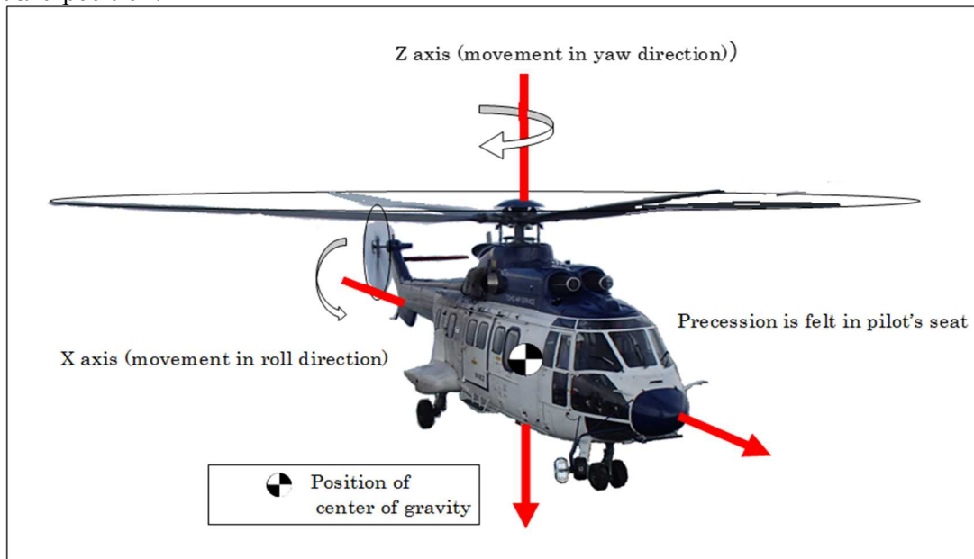
Figure 31: Unstable relation between lateral vibrations and rotating face of tail rotor
