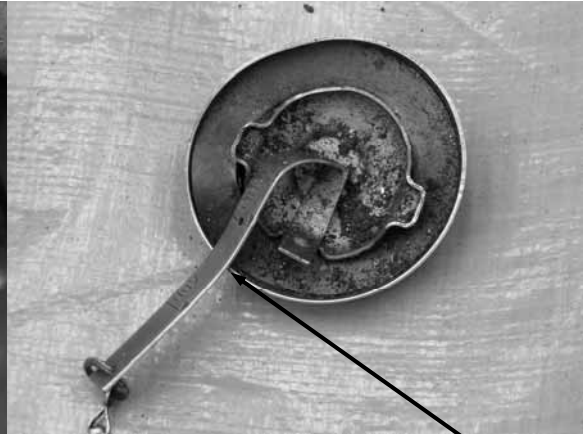
The Dipstick was bent after it was removed
