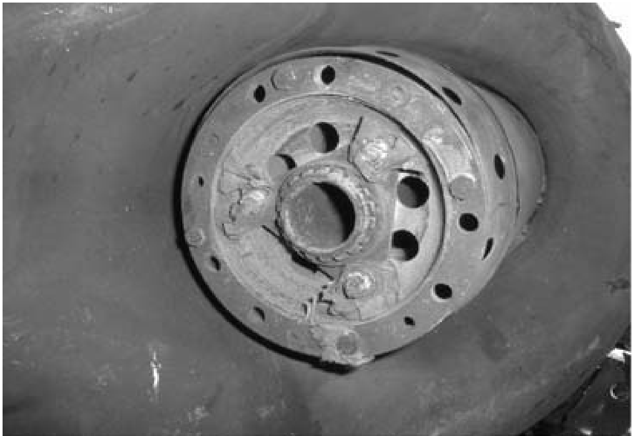
Photograph 5 No.1 Engine MGB Power Input (MGB Input Flector)
