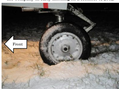
Nose landing gear of the Aircraft (Photographed by the Company in early morning on December 9, 2012)
