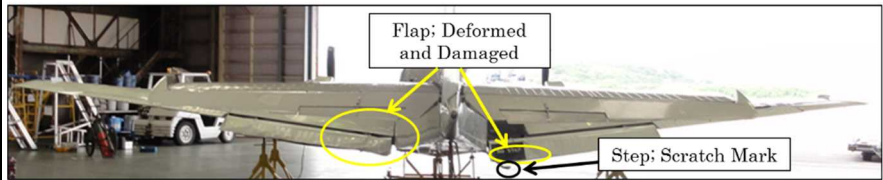
Photo 2 Damages of the front and rear
