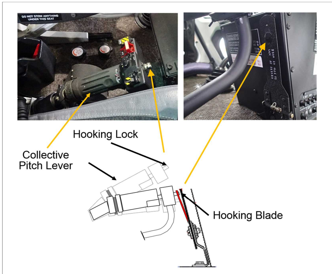
Figure 4 The Lock of Collective Pitch Lever
