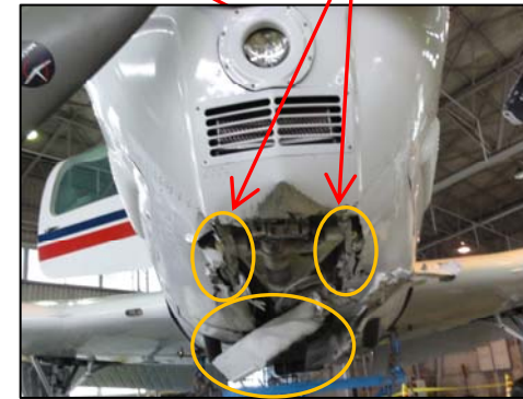
Deformation damaged nose gear door
