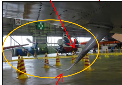
Black scratch marks on the VHF antenna support
