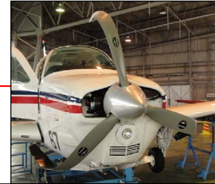
Bent propeller blades rearward
