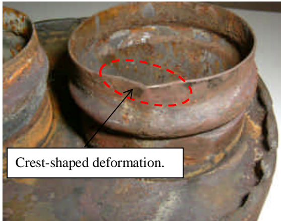
Right front connection pipe and the state of the clamp
