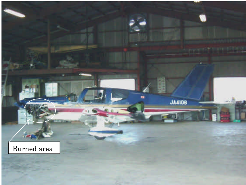
Photo 2 Lower Left Area of the Burned Engine
