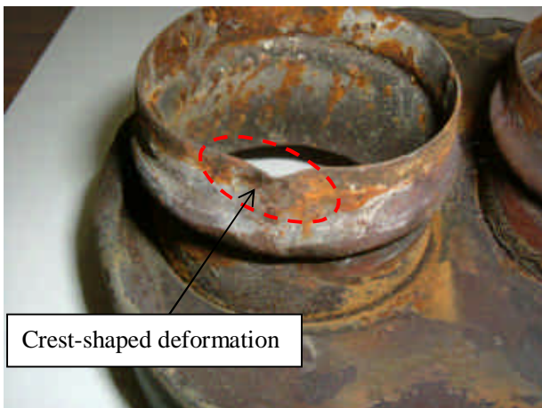
RH rear connecting pipe and the state of the clamp
