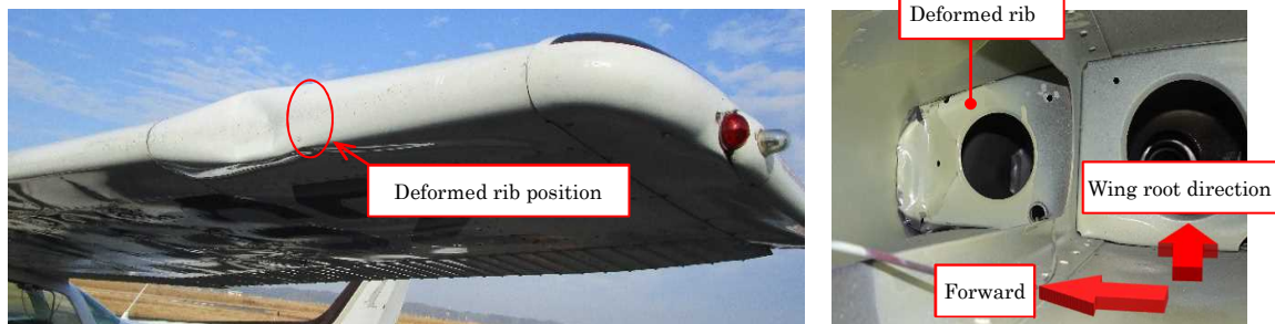
Figure 1: Damaged position of the accident aircraft (The right figure shows inside of the left wing taken from wing tip side)
