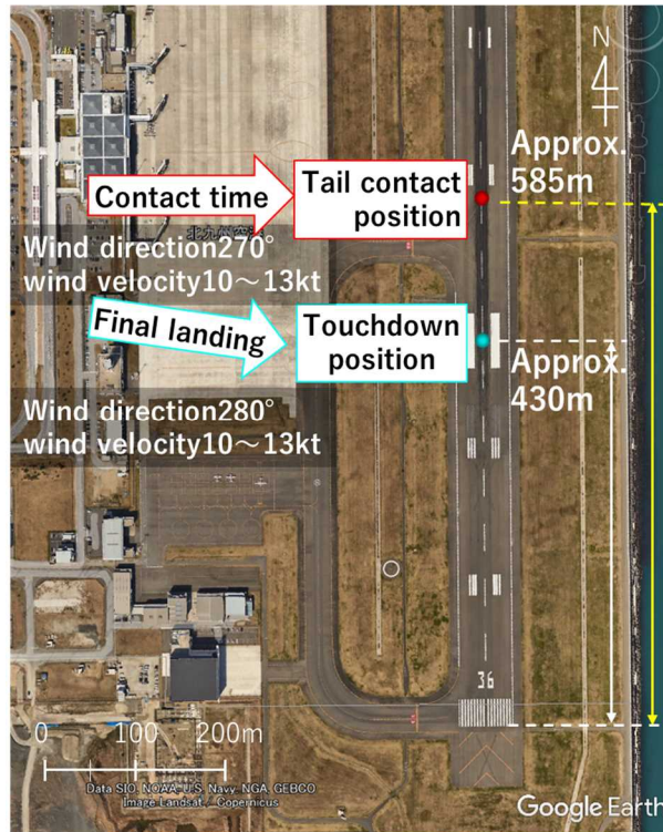
Figure 3 Contact (Touchdown) position
