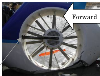
The edge of the through hole of Fenestron which the Rod had contacted
