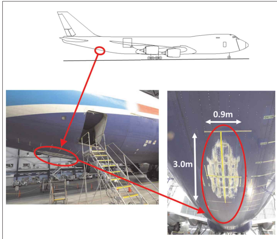
Figure 5: Conditions of damaged airframe
