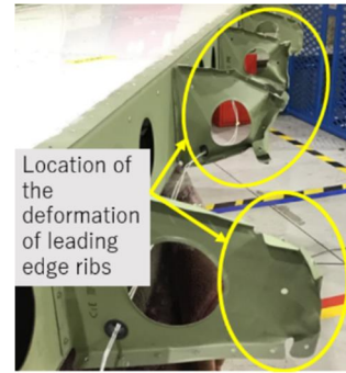
Figure 3: Location of Damage (Leading Edge Ribs)
