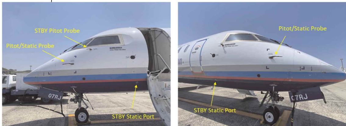
Figure 5: Pitot/Static Probe Installation Layout
