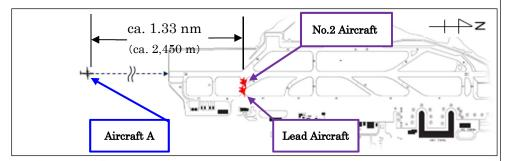
Figure 6: Position of Aircraft A when No. 2 Aircraft vacated runway
