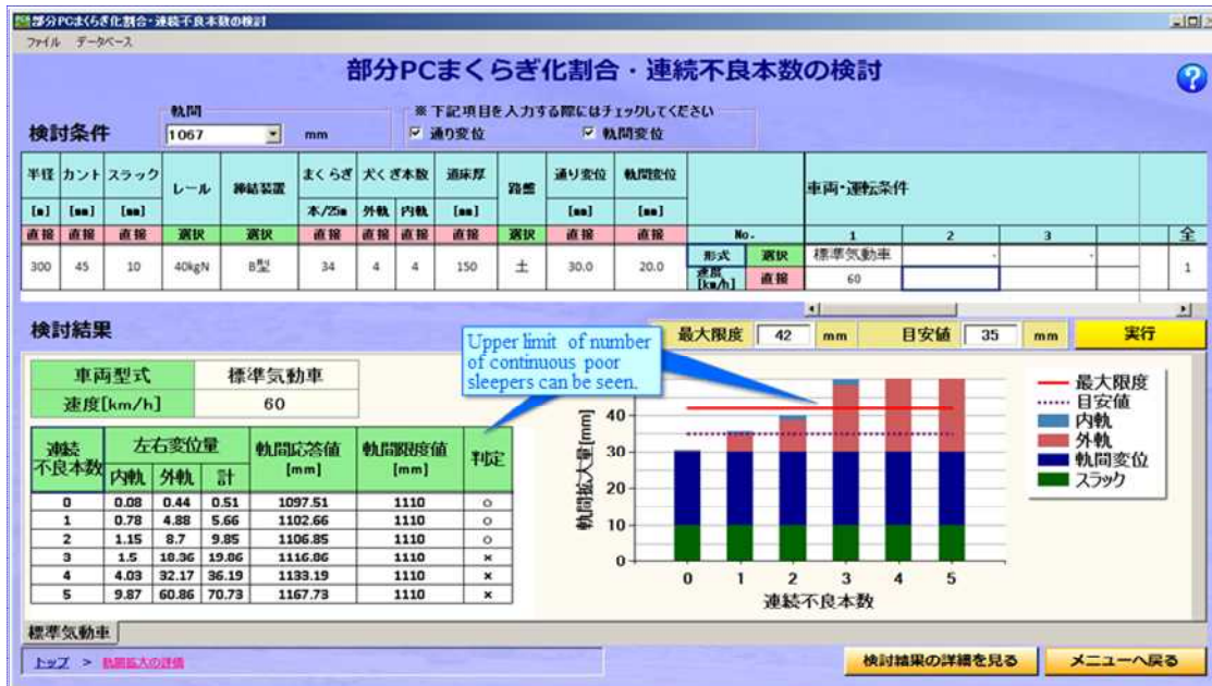
Display indicating the investigated results of the ratio of partially replaced PC sleepers.
