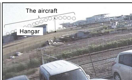
Cases of estimation based on visual images obtained are an entry angle from an aboveground target, left, a flying speed from the distance and time of flight, center, and a height of flight above the ground, right.
