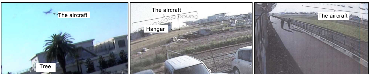
Cases of estimation based on visual images obtained are an entry angle from an aboveground target, left, a flying speed from the distance and time of flight, center, and a height of flight above the ground, right.
