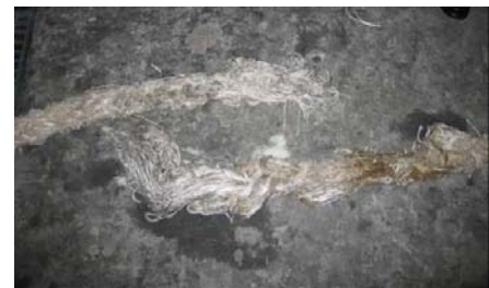
The Broken part of the Line
