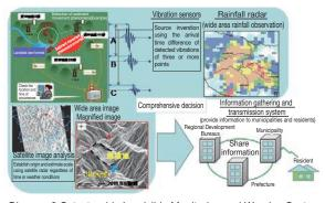
Diagram 3 Catastrophic Landslide Monitoring and Warning System Source) MLIT catastrophic landslides, the development of catastrophic landslides monitoring and warning systems<sup>Note</sup> (Figure II-10-1-3 Diagram 3) are being furthered to contribute to rapid emergency restoration measures as well as the prevention and mitigation of damages through appropriate warnings and evacuations.
