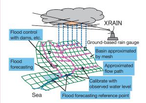
Diagram 2 flood prediction by distributed hydrological model Source) MLIT
