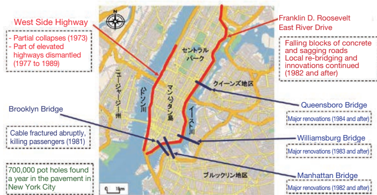
Bridge Damage Accidents in Manhattan Island in the 1980s and Major
