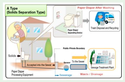
Three options are being considered as methods to accept soiled disposable diapers in the sewers, taking into consideration the local characteristics and the condition of the sewer facilities:
