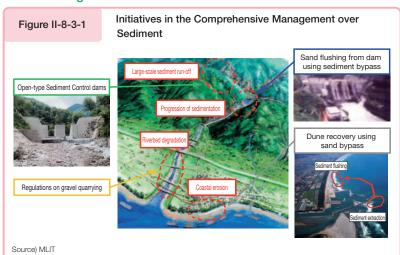
formulating comprehensive sediment management plans for effective sediment management and building sediment control dams, building open-type sediment control dams so that sediment can be effectively washed downstream, improving existing sediment control dams, creating an effective flow of sediment by sediment bypasses for dams, and recovering of sandy beaches by such methods as appropriate sand and gravel extraction of the waterways, sand bypass and littoral nourishment.
