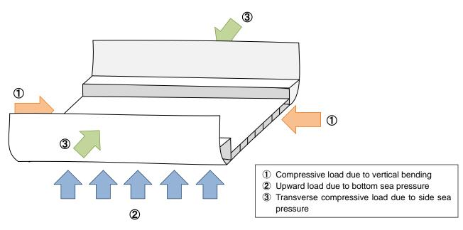
Figure A2-1 Load acting on Double Bottom Construction of Container Ships
