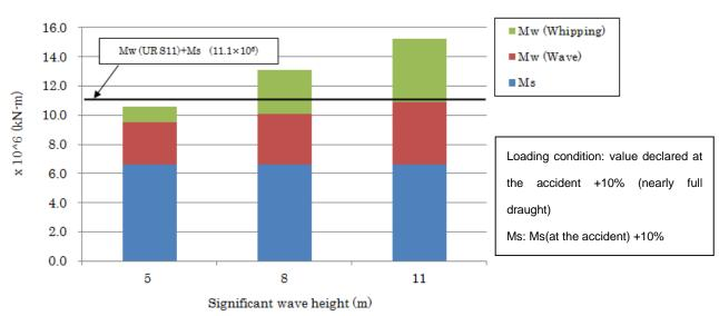
Ship(1) (The Ship) Vessel Speed 15 (knots) Mean wave period 12.5 (s) Head sea
