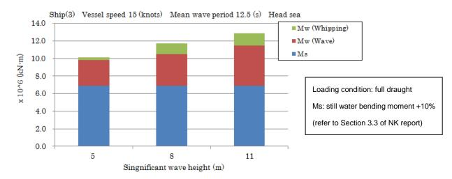
Figure 4.3.1 Example of the effect of acting loads (ship speed is constant)
