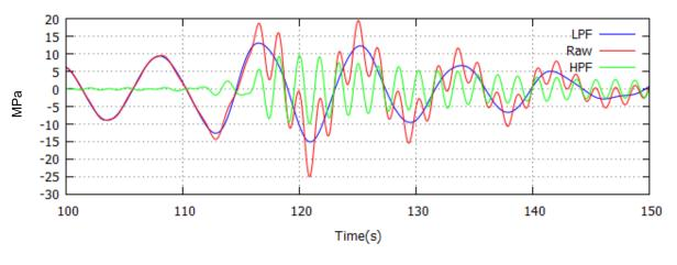
Figure A4-4 Longitudinal direction stress on the bottom shell plates
