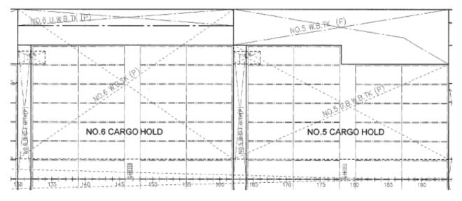
Fig 1.3.3 Tank Top Arrangement of No.5 & No.6 Cargo Holds (Port Side)
