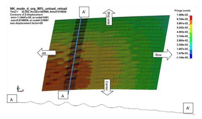
Maximum deformation 17.01 mm (double amplitude quantitative, deformation between longitudinal stiffeners would be about half of this double amplitude)
