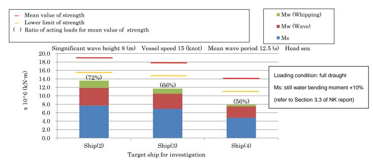
Figure 3.3.1 Ship structural strength and acting loads for large container ships (other than The Sister Ships)
