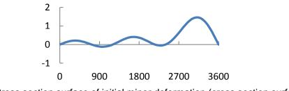
Figure A3-1 Cross section surface of initial minor deformation (cross section surface: mm)
