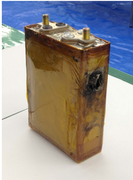
Cell 5 (Rupture disk was ruptured)
