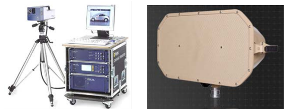
Photo. 2.1 SLDV (Polytec Corp., PSV400-H4) & LRAD(LRAD Corp., LRAD-300X)
