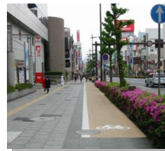
Bicycle track within sidewalk visually segregated from pedestrians by road marking
