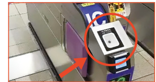
Ticket Turnstiles with QR Scanning Feature
