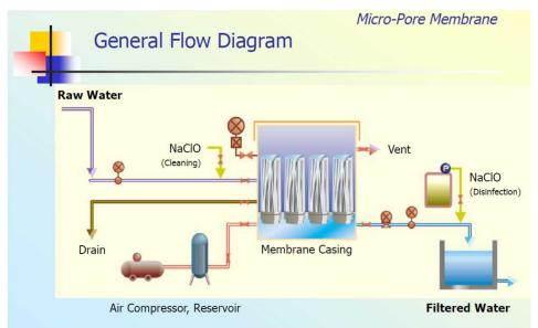
Conceptual diagram of a membrane filtration plant
